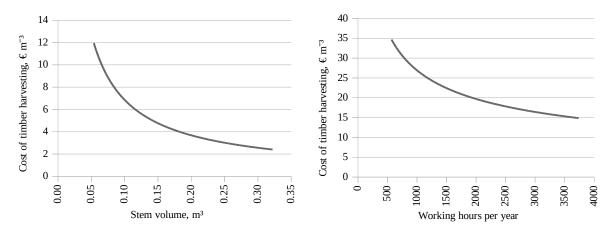
Fig. 2. Stem volume and harvester utilization rate impact on timber harvesting costs
